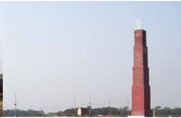
Zigzag chimney of Brick Kiln
